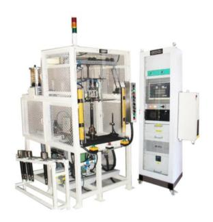
The Long Stem Tulip test systems is to test the weld bonding defcets. The Test Mechnism will have probe boom having probe arrangement to scan the test area. The probe will be placed on the head of the Job & then job will rotate for scanning.
