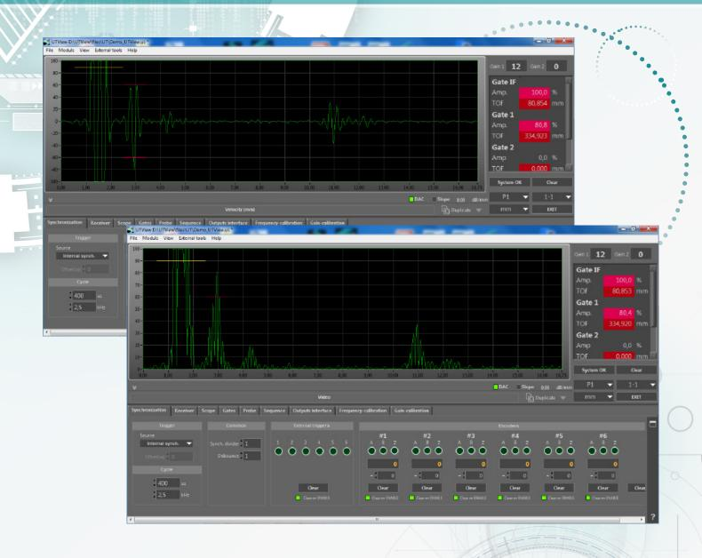
UTVIEW is the API's delivered with all Socomate International's products, compatible with both conventional and PAUT instruments. The software provides an A-scan view and allows to set all UT parameters.
