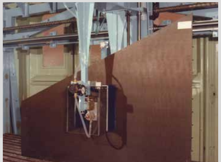
Water jet with squirts mounted on gantry scanning UT system for large composite structures in production
