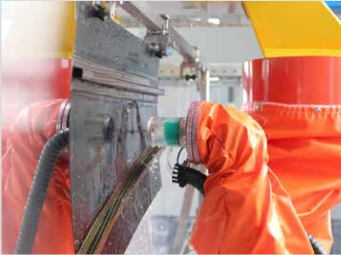
Squirters mounted on dual robot UT system
