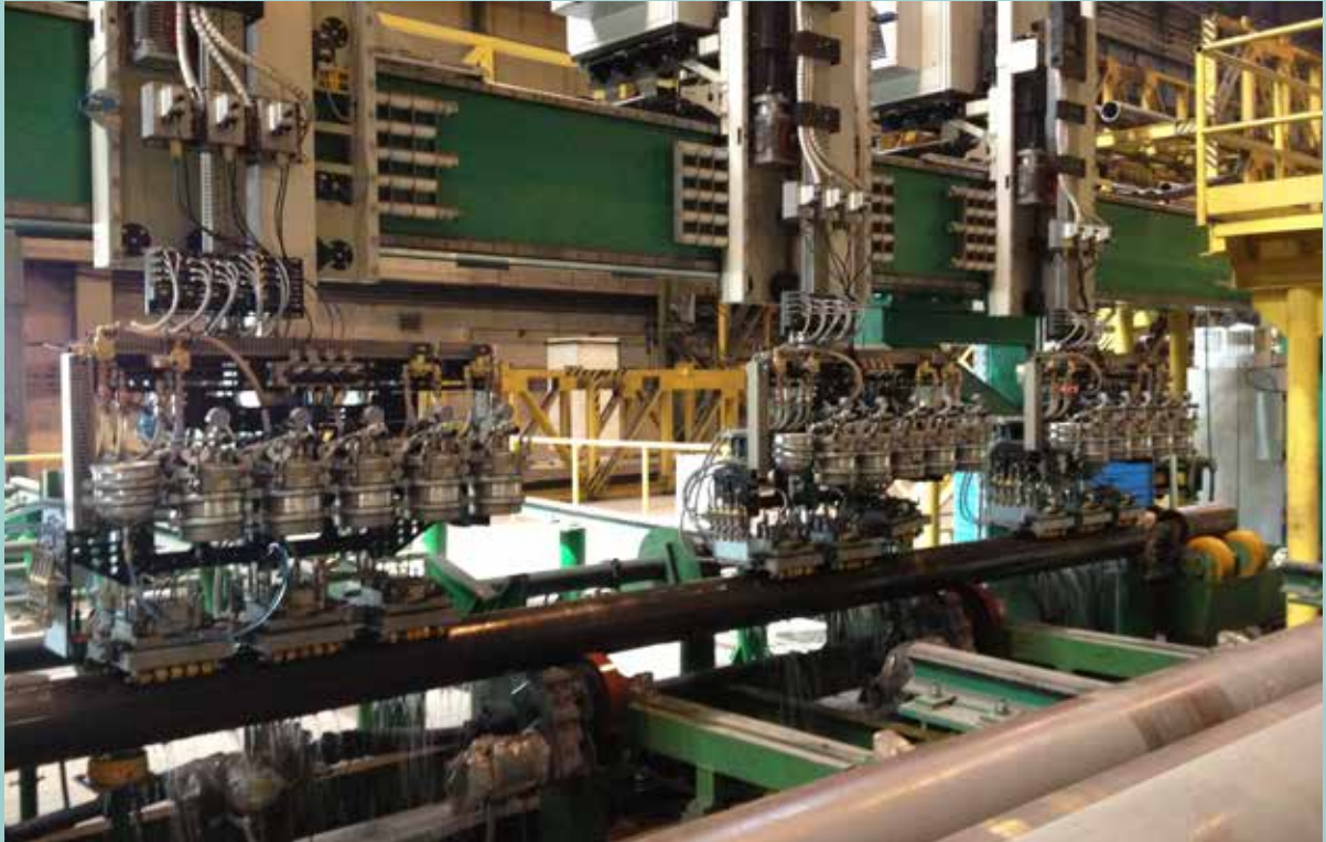
Full body UT inspection bench with FFAST Phased Array technology for OCTG
