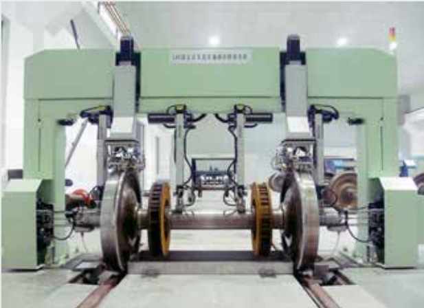
Wheel-set inspection in Work Shops without dismantling wheels from axles
