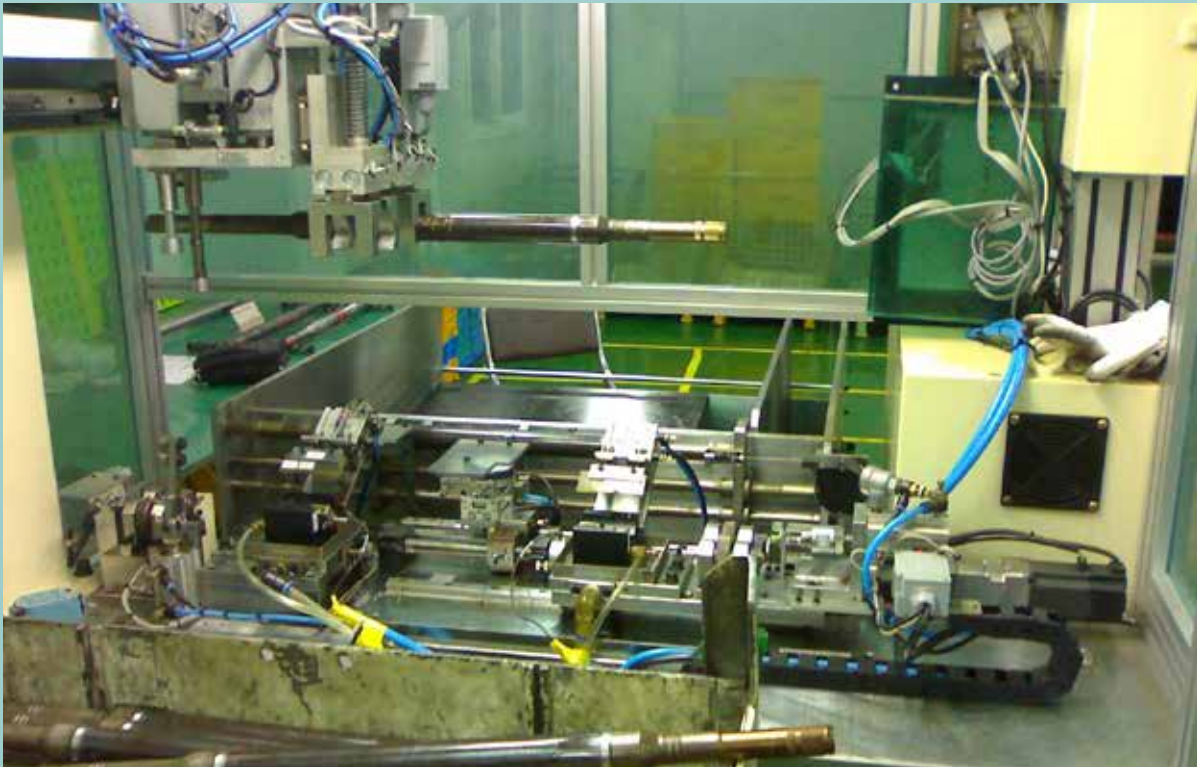
Car steering rods with semi automatic system for the eccentricity measurement
