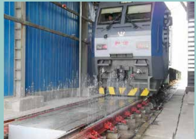
UT inspection of the wheels without dismantling the wheels set from the car
