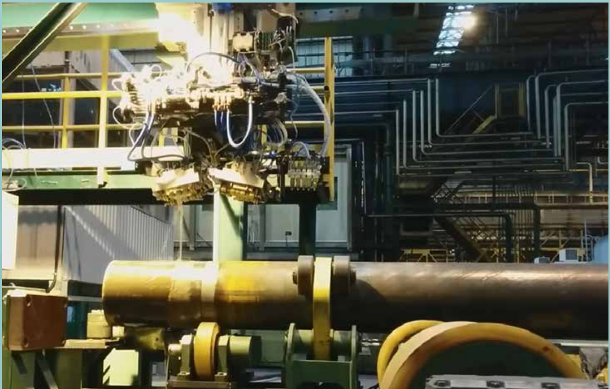
Inspection of tube extremities with FFAST Phased Array technology
