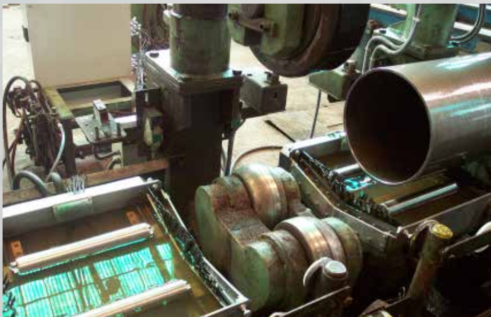
Flaw detection and wall thickness measurement for seamless tube in-line
