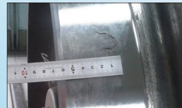
Defect in wheel rim
