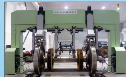
Wheel set inspection configuration
