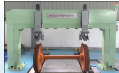
Wheel inspection configuration
