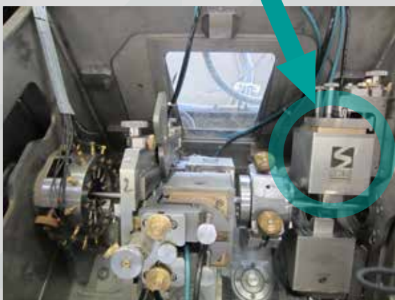
Alternative to rotary head by using e.Rota combined with FAAST Phased Array
