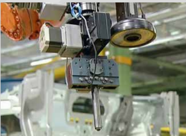
Spot weld testing in-line
