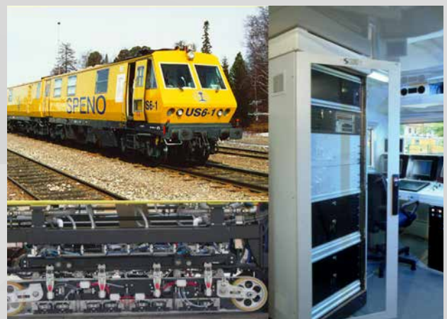
On-track rail inspection at 100km/h non-stop
