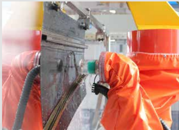
Composite testing with squirters robots
